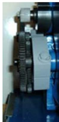
when thread cutting is wanted remove the FF mod and install the banjo with the appropriate gears mounted.
