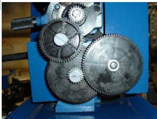
An end view and front view show the finefeed mod in use. Use the lathe this way except
