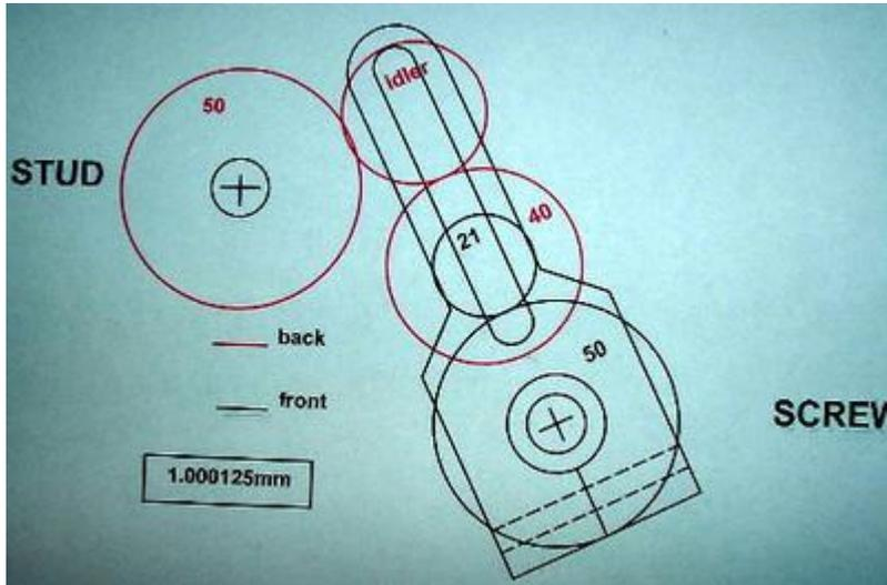
The drawing shows how the gears are arranged on the banjo while the picture shows it in place, ready to operate.
