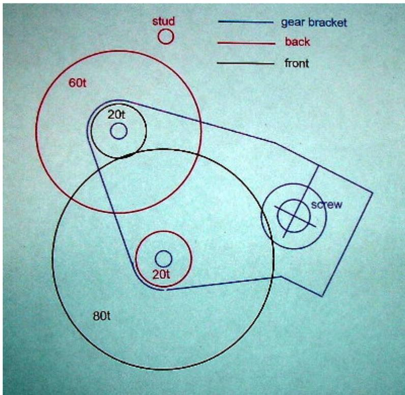
The fine feed module can be made of 3/8 aluminum or from thicker plastic as in the pictures above.
