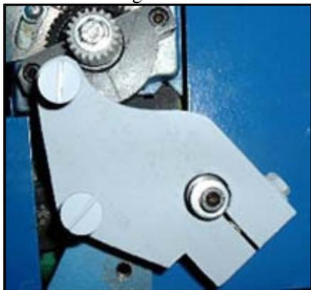
Probably the most useful feed device would be a variable speed motor type since the rate can be set as preferred, but it can be complex and is usually in the way. A cartridge type module, dedicated to providing a suitable feed rate for a nice finish, can be easily built. The fine feed module reduces carriage rate by about a factor of 4 from the original minilathe setup. When threading is to be done, the cartridge is removed intact and a simple banjo with change
