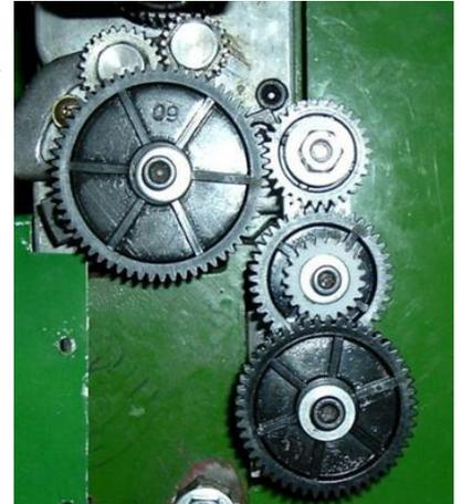
The idler gear is needed with a few threads, most don't need it so you could make one gear shaft to start and make the
